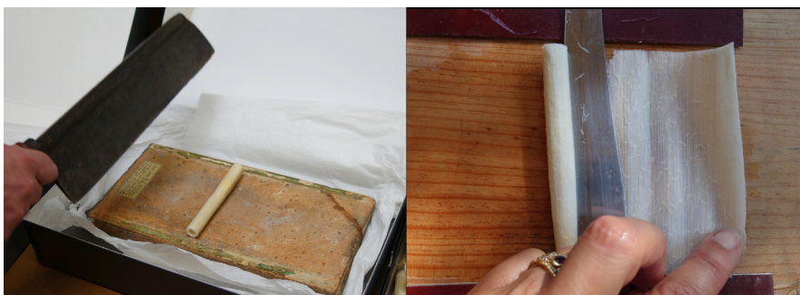
Fig. 15 Tools for pith paper manufacture from the Economic Botany Collection, Royal Botanic Gardens, Kew, and experiments on papyrus pith with a similar technique.
