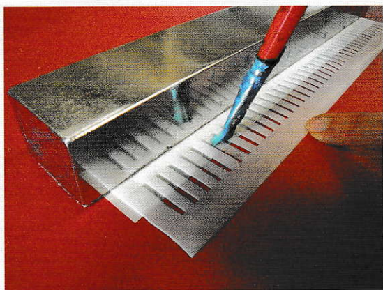
FIGURE 12 Teflon stencil plate used for pasting out hinges with micro lines. A blue food colouring was added to the adhesive to make the pasted lines visible
